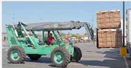
This is an example of a portable self-propelled rough terrain forklift that is typically transported to the job site. It is mounted on a carrier to the back of a truck/trailer and is used to unload heavy items from the truck/trailer at the job site. Note that not all truck/trailer mounted forklifts are rough terrain forklifts.
