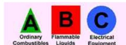
This is the new style of labeling that shows this extinguisher may be used on Ordinary Combustibles, Flammable Liquids, or Electrical Equipment fires. This is the new labeling style with a diagonal red line drawn through the picture to indicate what type of fire this extinguisher is NOT suitable for. In this example, the fire extinguisher could be used on Ordinary Combustibles and Flammable Liquids fires, but not for Electrical Equipment fires.
