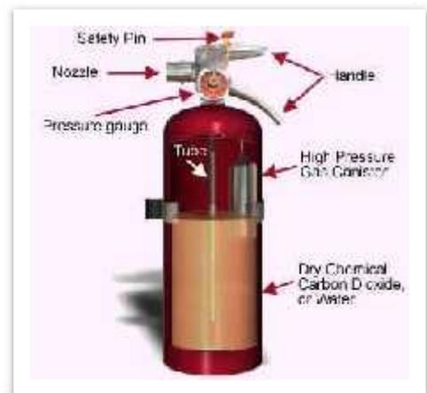
All portable fire extinguishers must be approved by a nationally recognized testing laboratory to verify compliance with applicable standards. Equipment that passes the laboratory's tests are labeled and given an alpha-numeric classification based on the type and size of fire it will extinguish.
