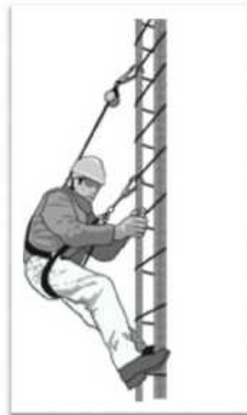
A positioning-device system with a self-retracting lifeline.
