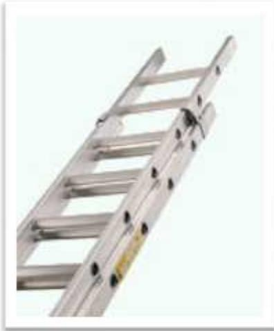
Extension ladders offer the most length in a general-purpose ladder. They have two or more adjustable sections. The sliding upper section must be on top of the lower section. Made of wood, metal, or fiberglass. Maximum length depends on material. Supports only one worker.
