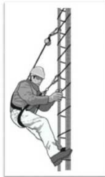
*A positioning-device system with a self-retracting lifeline.*
