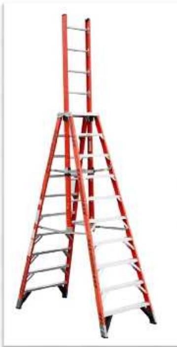
Trestle ladders have two sections that are hinged at the top and form equal angles with the base. Used in pairs to support planks or staging. Rungs are not used as steps. Length cannot exceed 20 feet.
