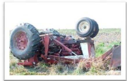
Tractor without ROPS at scene of overturn.
