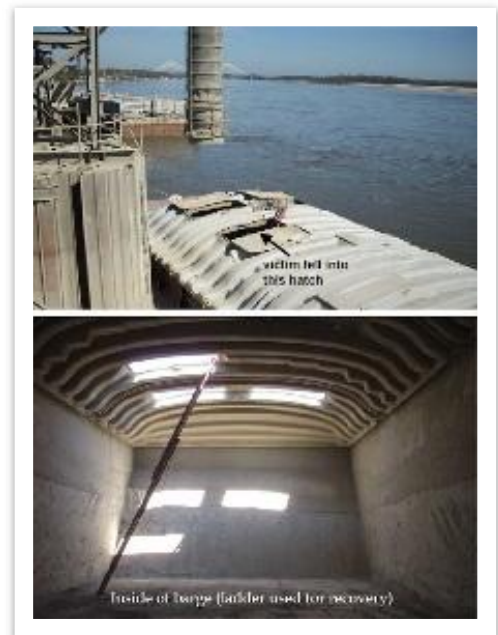
Worker suffers a fatality from falling through hatch in barge.
