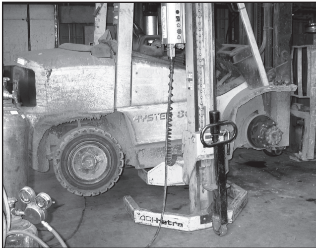
This forklift truck, raised for repair work, has potential energy.
